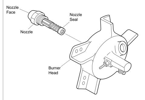
Figure 17 - Removing Nozzle, 150,000 BTU/Hr Model
